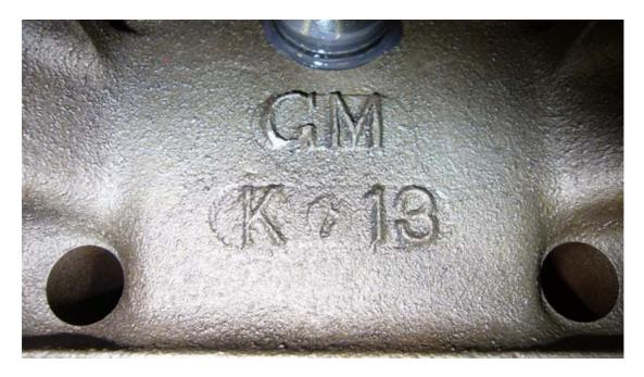
This dating system, used on mid-60s through to early 70s cars, uses a letter and number to designate the month and day a part was cast. The letters run from A through to M, bypassing the letter "I" and decode as follows:
