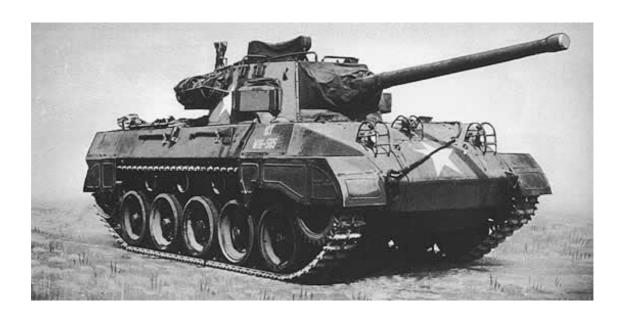
"Buick's Hellcat, Model M-18 had a range of 105 miles and weighed 17 tons. With its 9 cylinder 400 horsepower engine, the Hellcat boasted an excellent power-to-weight ratio making it the fastest tank of World War II with a top speed of 55 mph. The Hellcat sported maximum maneuverability, high firepower and all steel, centre guided tracks. It could smash tanks at several miles. The Hellcat proved superior to latest versions of the German Tiger Tank in actual battle and was 30 mph faster!
